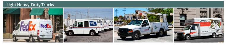
Light heavy-duty trucks are smaller trucks weighing between 14,001 lbs and 19,000 lbs. Examples include small delivery trucks, large vans, work/utility trucks, etc.
