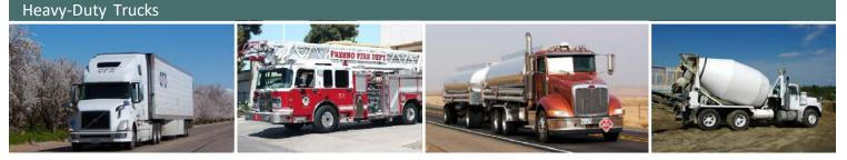
Heavy-duty trucks are the largest class of trucks weighing more than 33,000 lbs. Examples include dump trucks, concrete pump trucks, refuse hauling, long-haul, port/drayage trucks, charter buses, emergency trucks, etc.
