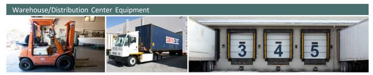
Equipment used to move objects short distances for warehouse or freight operations. Examples include forklifts, yard goats, etc.
