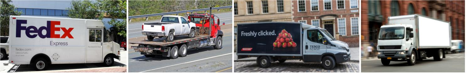
Medium heavy-duty trucks, weighing between 19,501 lbs and 33,000 lbs, are larger than light-duty trucks but smaller than heavy-duty trucks. Examples include, delivery trucks and tow trucks.
