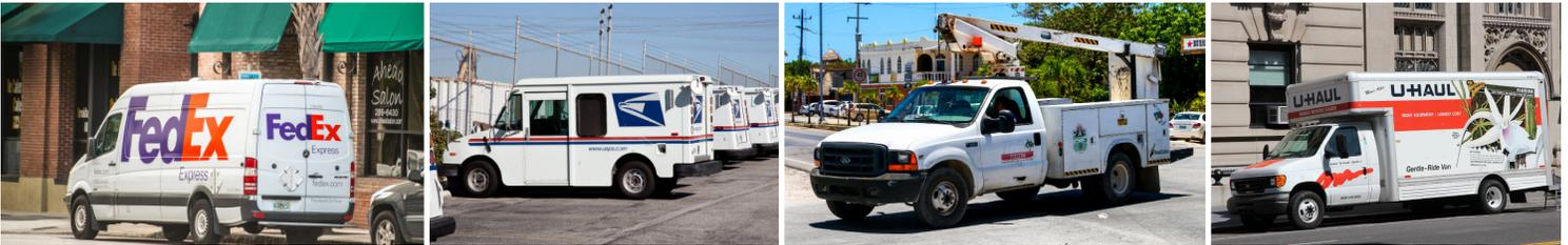
Light heavy-duty trucks are smaller trucks weighing between 14,001 lbs and 19,000 lbs. Examples include small delivery trucks, large vans, work/utility trucks, etc.
