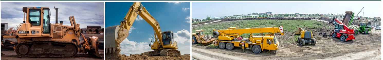
Equipment specially designed for executing construction tasks, most frequently ones involving earthwork operations. Examples include loaders, excavators, bulldozers, cranes, etc.
